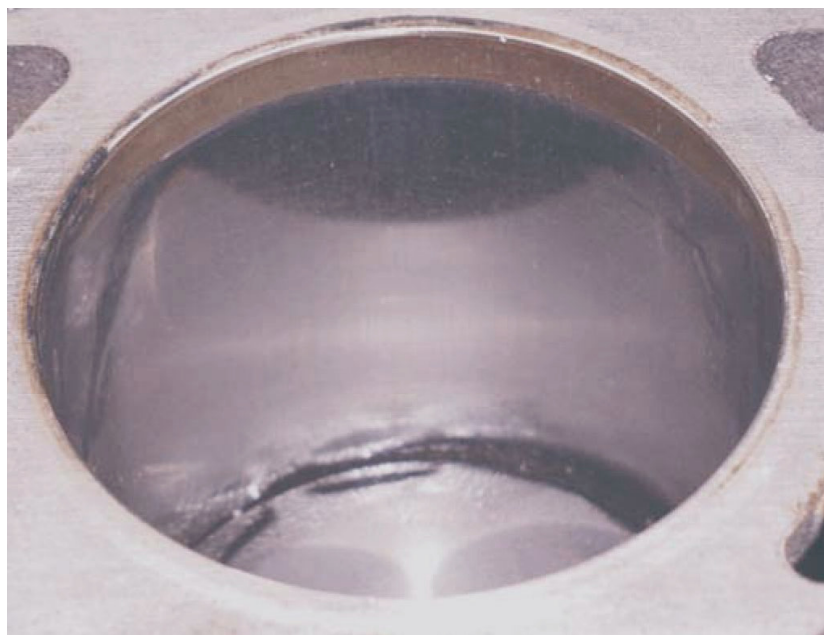
Figure 5-1: Digital recording of the Ford Escort's engine block following treatment (alterations to the surface are clearly visible)
